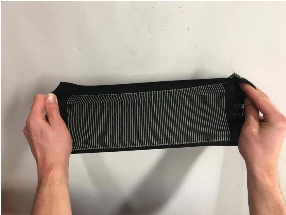
Stretchable and stable: Demonstrator of a textile heater. Photo: DITF
