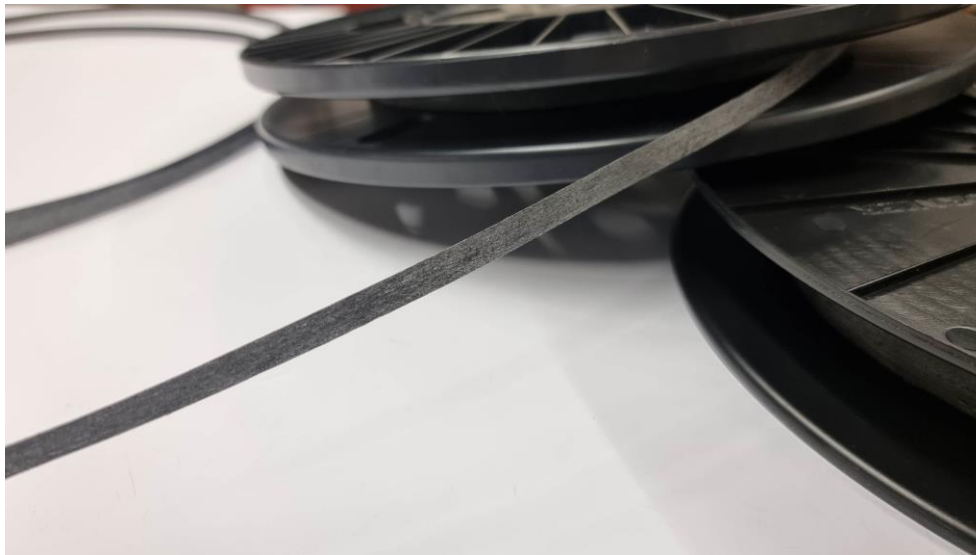
Tapes for high-performance applications made from recycled carbon fibers: Photo: DITF.
