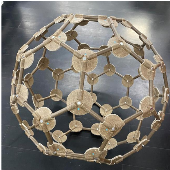
Final structure as buckyball with the developed nodes and pultrusion profiles. Photo: Carsten Fulland, Zenvision
