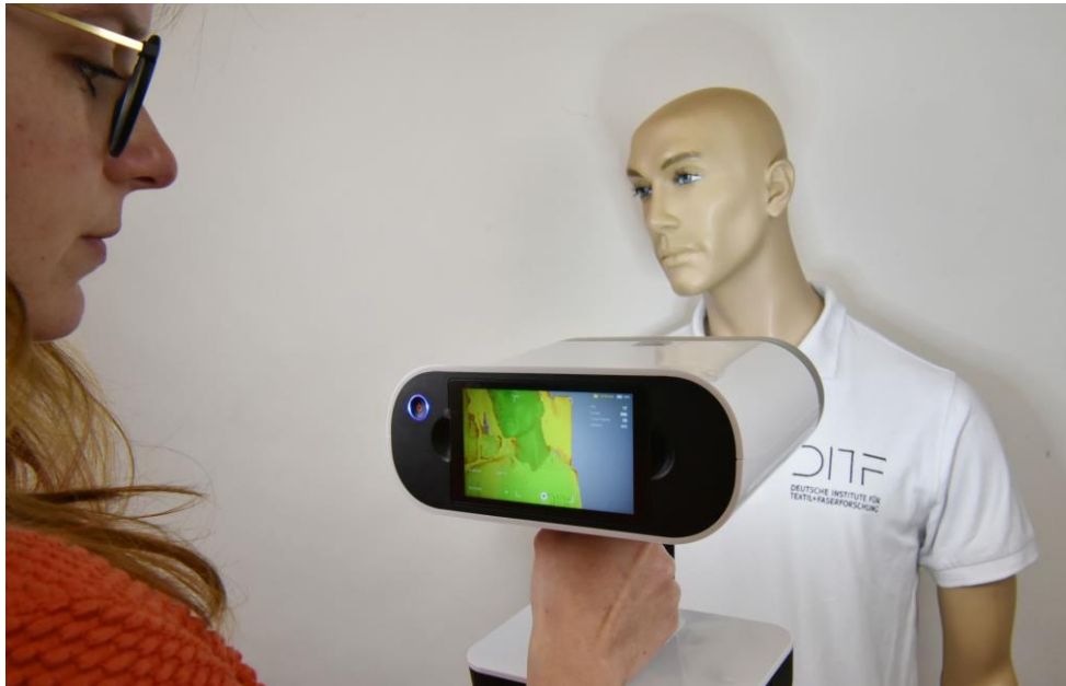
Hand-held 3D scanners can be used to digitize patient body parts as the basis for flexible textile orthoses. Photo: DITF
