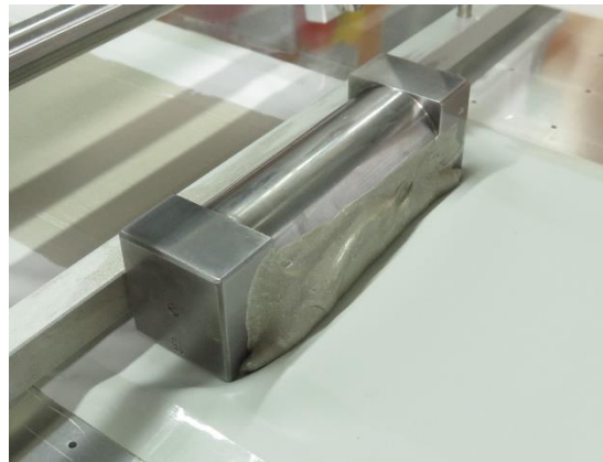
Image 02: Applying the conductive layer with a squeegee
