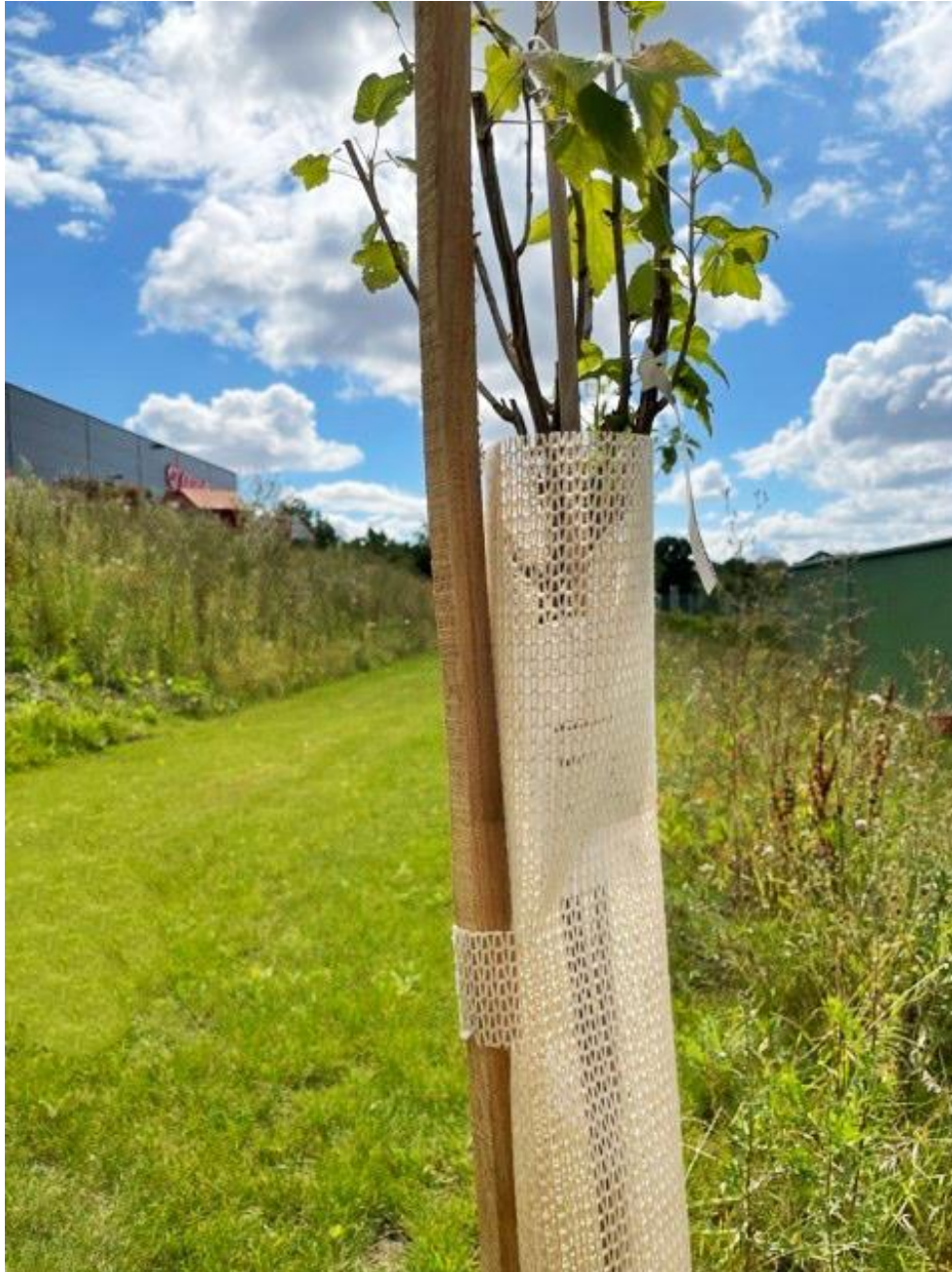
Tree cover made of yarn developed at the DITF in use. Photo: Buck GmbH & Co. KG
