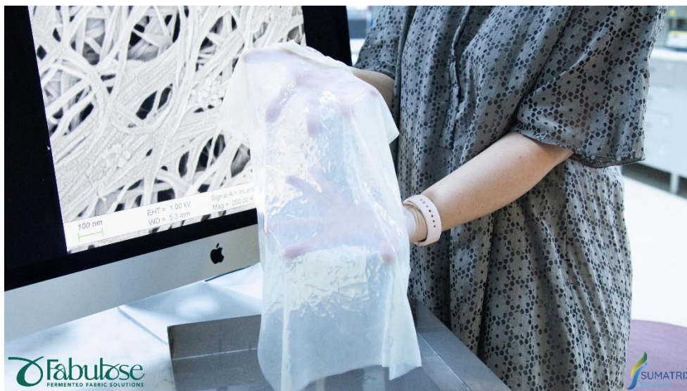
Bacterial cellulose film produced by Sumatrix . Photo: Source: Sumatrix Biotech (CC BY-NC 4.0)
