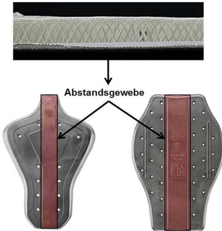
Photo 2: Manufactured textile-reinforced demonstrators for the back protector. Photo: DITF
