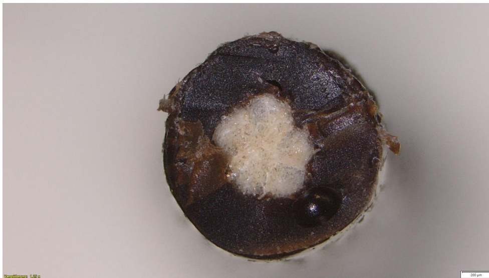
Cross-section of a cotton yarn coated with lignin by extrusion process. Photo: DITF
