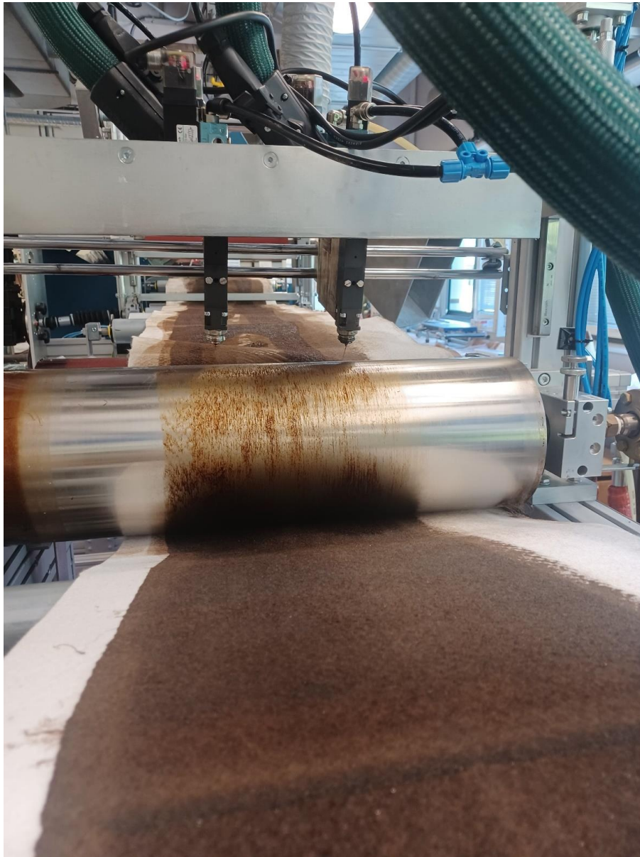
Nonwoven fabric based on cellulose, coated with the lignin compound as a protective layer against degradation in the soil. Photo: DITF
