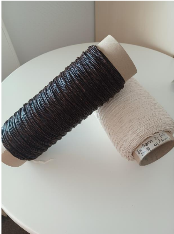
Cotton yarns: with lignin coating as a protective layer against degradation in soil and reference material without coating. Photo: DITF
