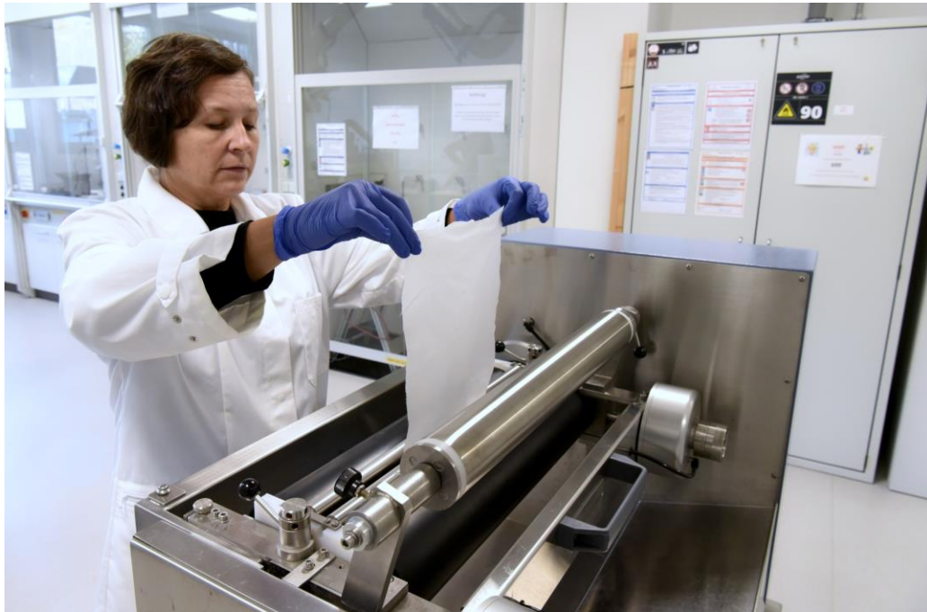
Finishing a fabric on a laboratory padder. Photo: DITF
