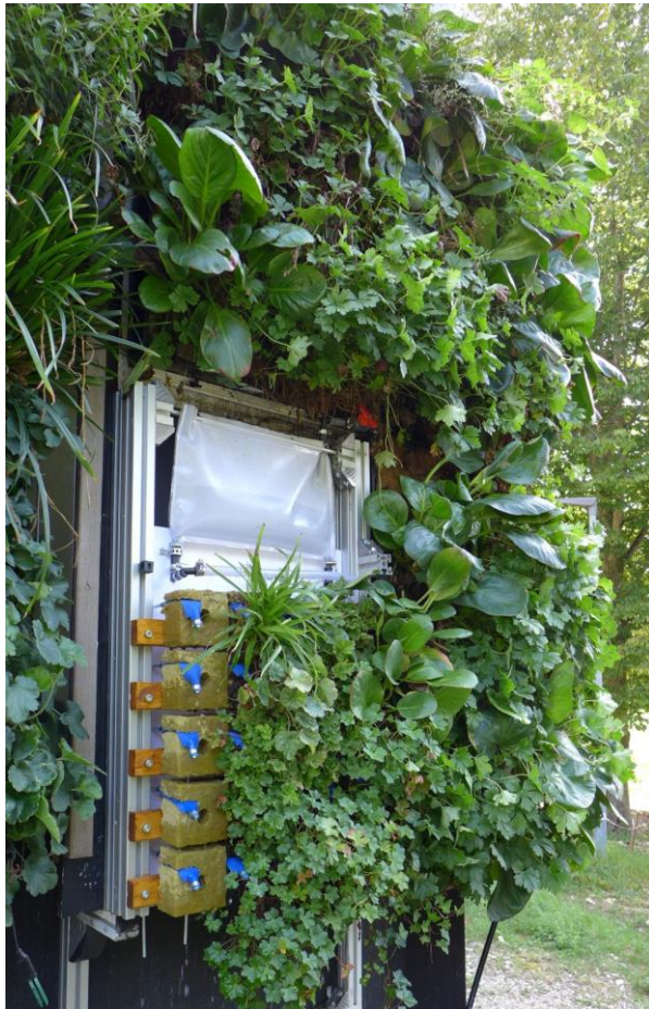
Outdoor demonstrator on the Research CUBUS. At the top is the textile water reservoir with all inputs and outputs and textile valve for rapid emptying. Below are the substrate blocks with integrated hydraulic textiles. Photo: DITF
