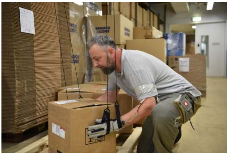
Moving heavy loads without physical strain using SensHand. Photo: DITF
