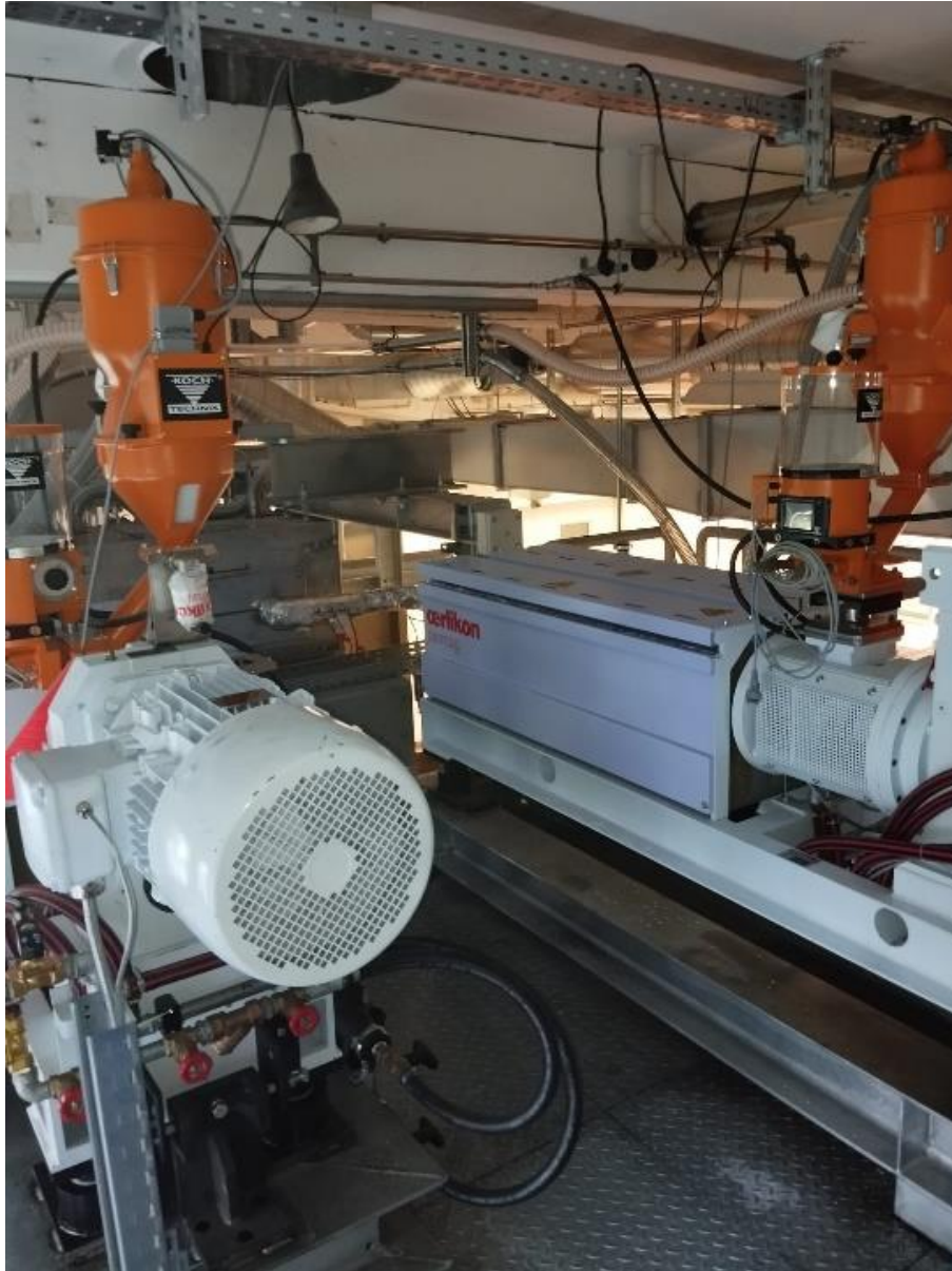
Pumps and extruder of the bicomponent BCF spinning system from Oerlikon Neumag. Photo: DITF.
