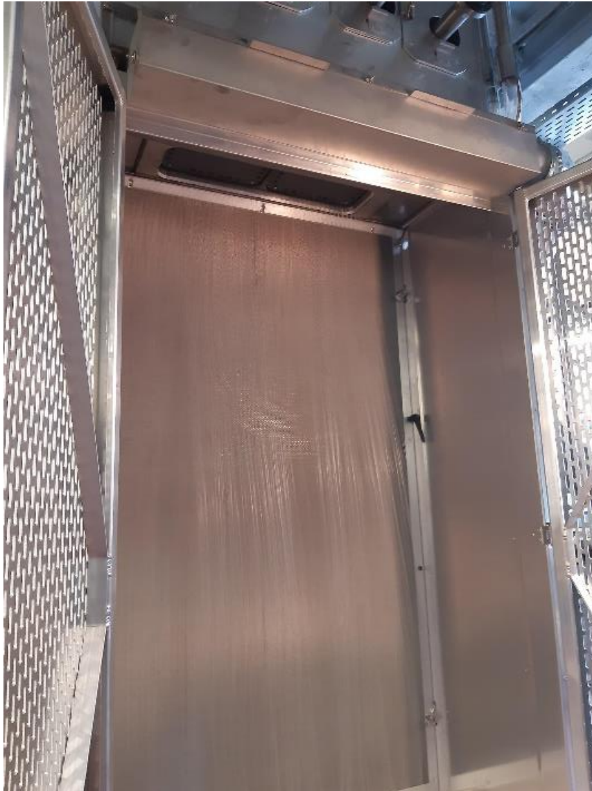
The spinning shaft of Oerlikon Neumag's bicomponent BCF spinning plant with the freshly extruded fibers. Photo: DITF
