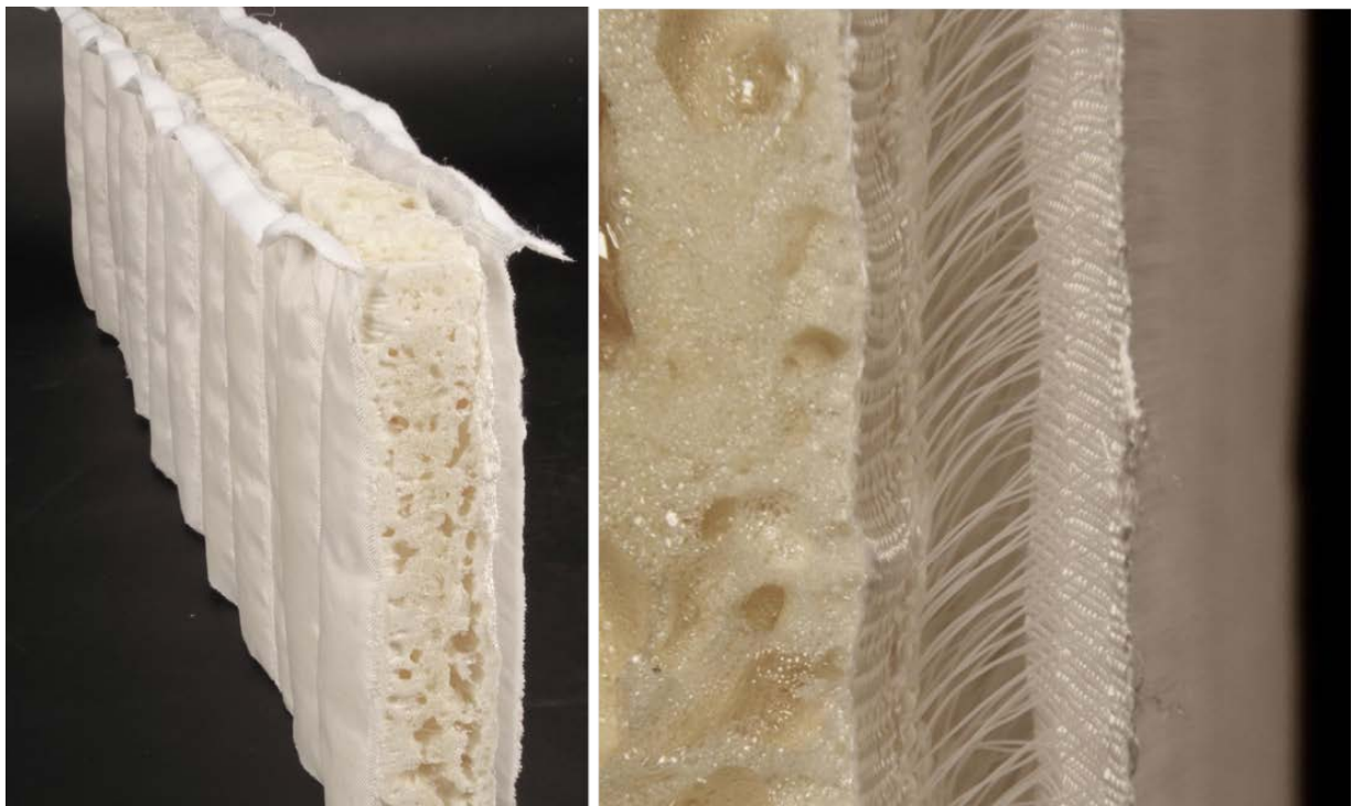
Image 2: spacer fabric, left horizontally and foamed manually with PU foam, on the right a section through the insulation- and rear ventilation level (photos: FRA-UAS)
