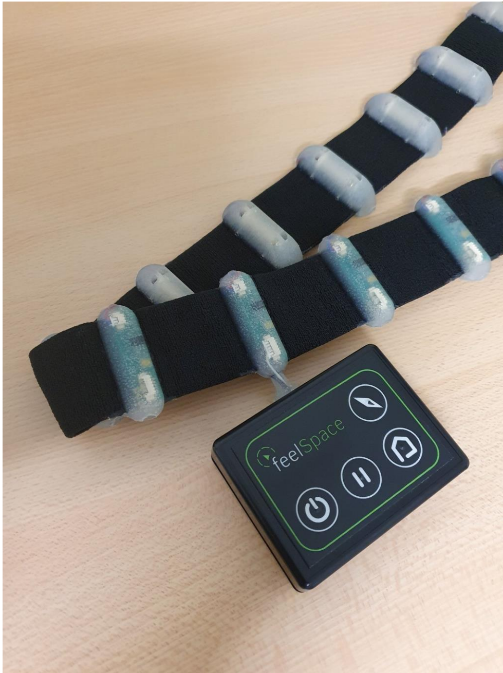
Demonstrator manufactured using ultrasonic welding. Photo: feelSpace
