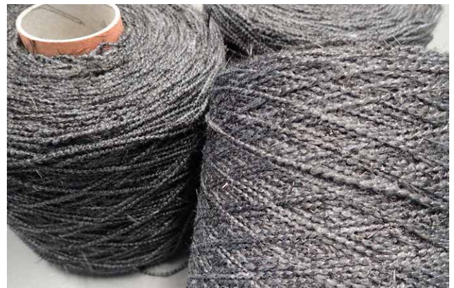
rCF/PA wrapped hybrid yarn
