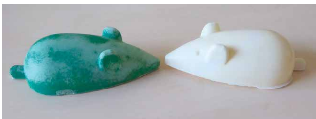
In-situ polymerized demonstrator components manufactured through rotational molding
