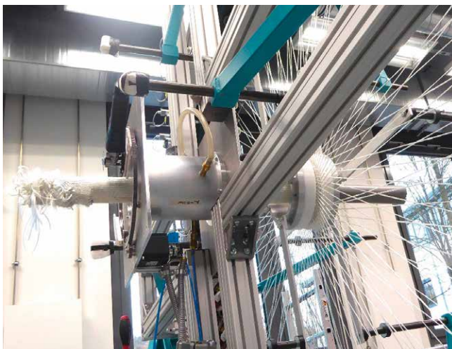
Braiding machine equipped with clamping and cutting devices
