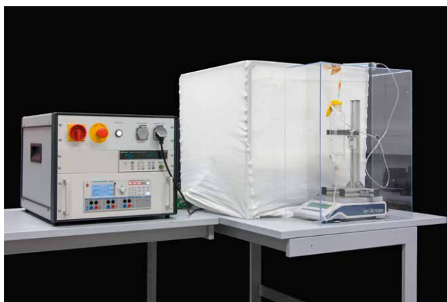
Thermal balance measurement setup (WMB)
