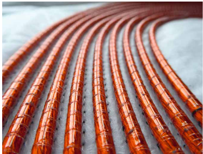
Copper coil embroidered on structural textile
