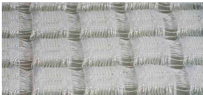
Spacer fabric that is filled quickly with foam and adaptive to bends
