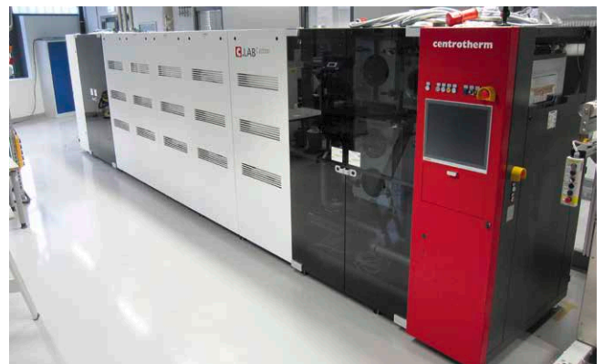
Novel low-pressure stabilization furnace at the DITF
