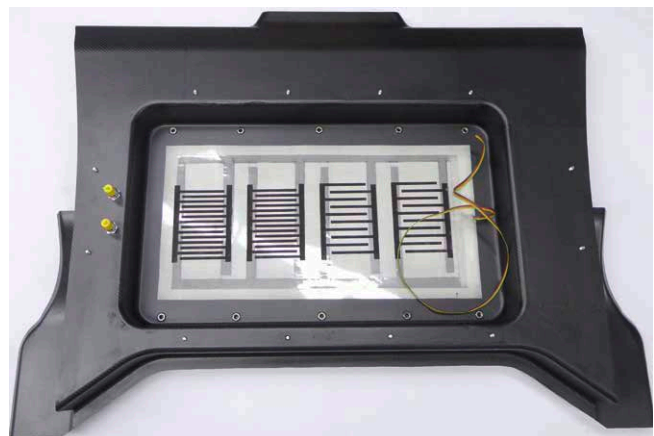
Rear floor with integrated inserts, water supply and printed humidity sensor
