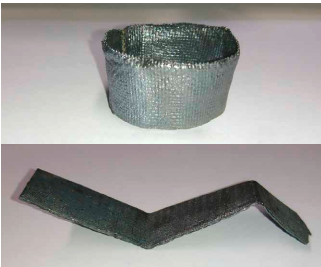
Fiber-reinforced ceramic composites made from pure cellulose composites in the shape of a Z-profile and tube
