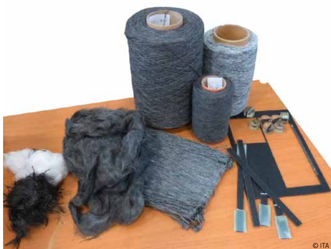
Products of the individual recycling process steps in the CarboYarn project
