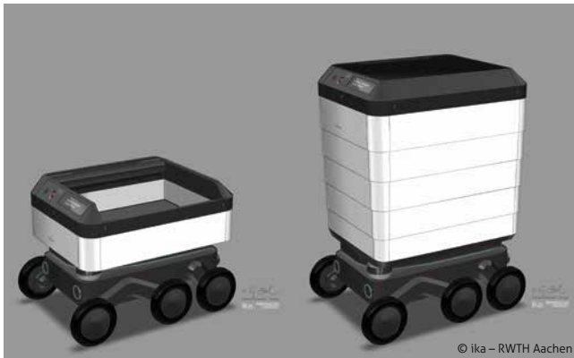
UrbANT with height-adjustable superstructure
