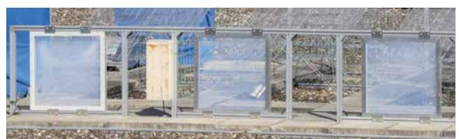
ETFE facade elements in the outdoor weathering facility at DITF
