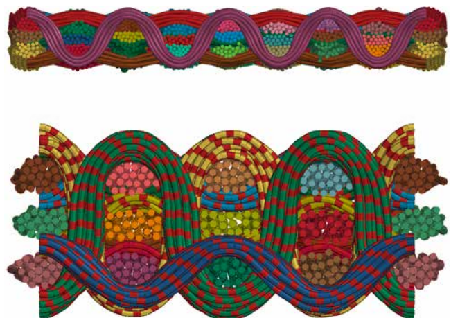
Generation of the meso-model of a 3D fabric
