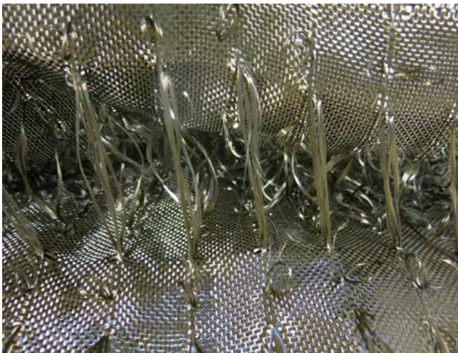
Basalt spacer fabric with pile thread spacing 150 mm
