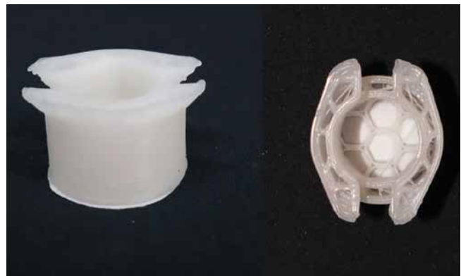
Multiwell insert with integrated cell carrier fleece
