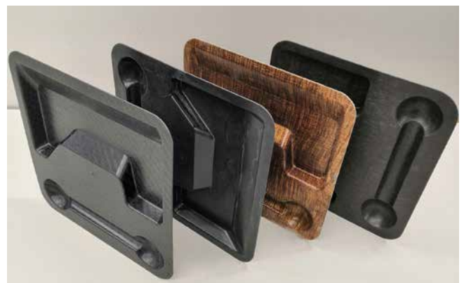
Demonstrator components made of different materials; from left to right: staple fiber fabric (rCF/PA6), nonwoven fabric (rCF/PP), viscose fabric (CV/CA), nonwoven fabric (rCF/PA6)
