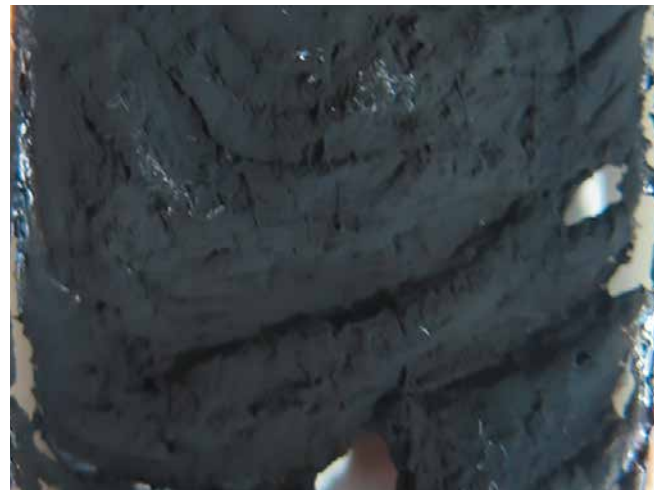
Cellulose phosphite coating after intumescence, coated substrate underneath is largely preserved
