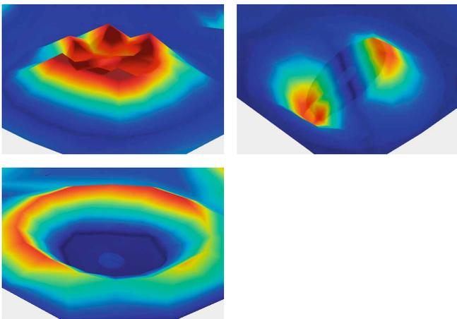
Three eigenmodes of the textile resonators
