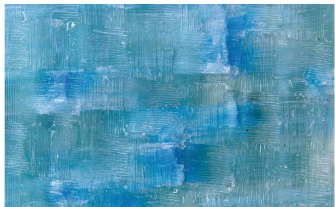
Self-healing glass fiber reinforced plastic thanks to storage depots made of hollow glass fibers
