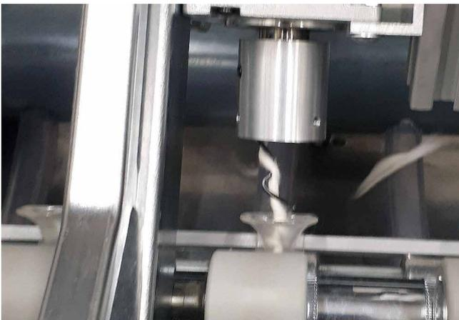
Twist offset element before the drafting system of a ring spinning machine
