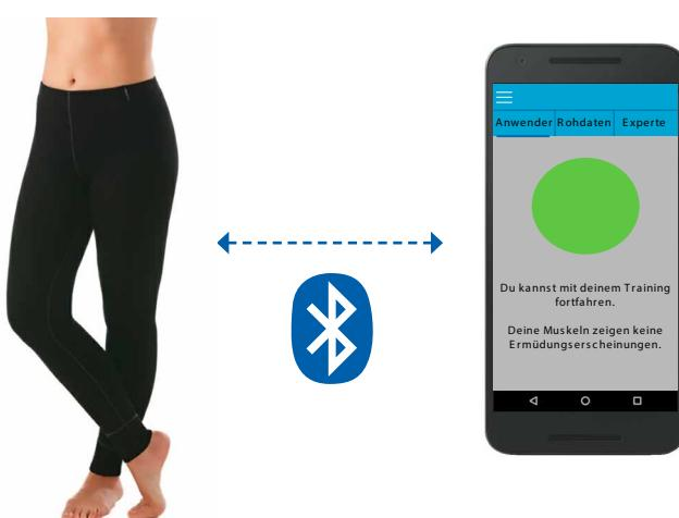
Sports trousers with real-time monitoring of muscle functions using electromyography
