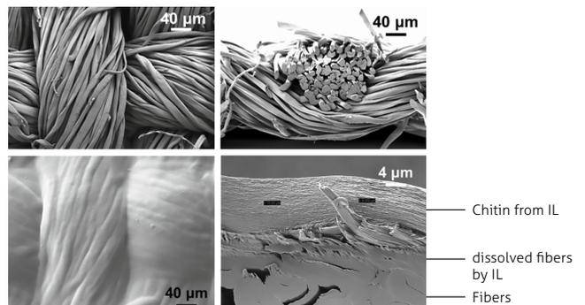
SEM images of uncoated cotton fabric (top) and cotton fabric with chitin coating (bottom)
