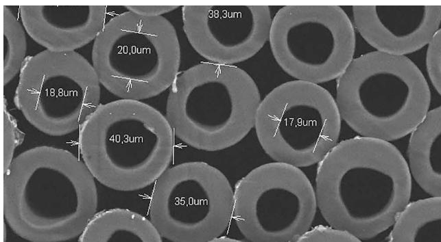
Cross sections of hollow fibers made of the biopolymer PLA
