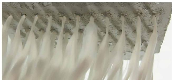
Cellulose filament yarns embedded in concrete
