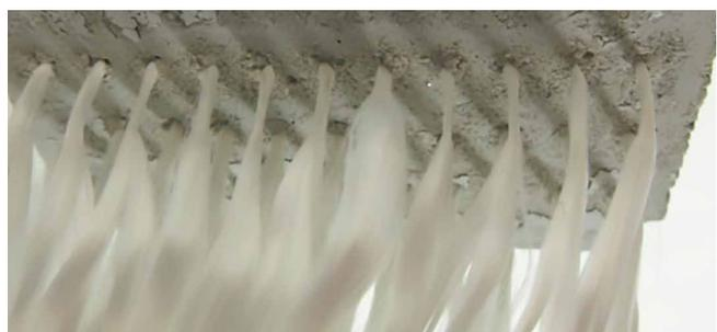
Cellulose filament yarns embedded in concrete
