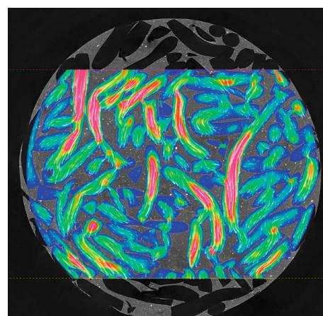
$\mu$ -CT Image with flow simulation of the interconnecting pores of the bone substitute material
