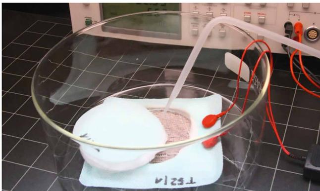
Determination of the moisture on the laboratory sample Wound covering with sensor yarns
