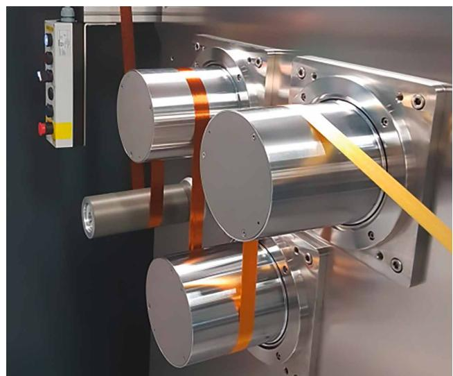
50 K polyacrylonitrile precursor at the outlet of the low pressure furnace
