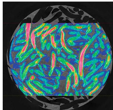
$\mu$ -CT Image with flow simulation of the interconnecting pores of the bone substitute material
