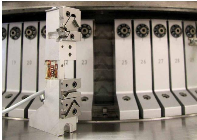
Modified lock segment for measuring the sinking force
