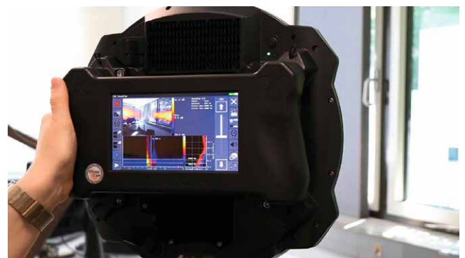
Absorption effect of the ecological absorber panel of the DITF shown by means of an acoustic camera
