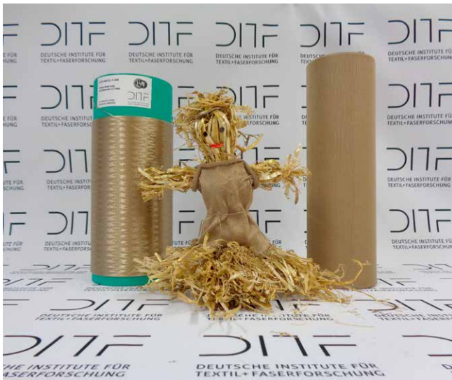
From straw to sustainable textiles – filaments and knitted fabrics made from straw pulp
