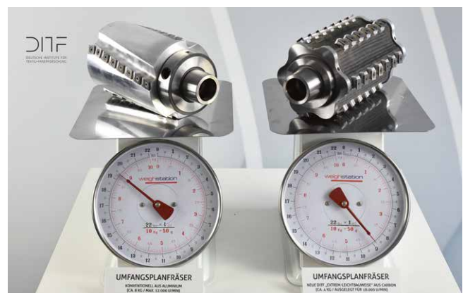
New extrem-lightweight planer head – 50% lighter and 1.5 times faster than the reference aluminium peripheral milling cutter (ThinkIng Award May 2022)
