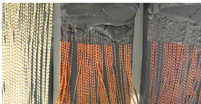
Adhesion of polyamide 6.6 to rubber: without adhesion promoter (left), with RFL dip (center), with HMF dip (right)
