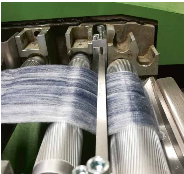
Developed fiber guiding element with optimized position in the drafting system of a draw frame
