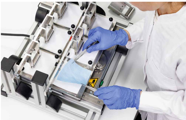
ReBa²-testing device for determining the bacterial penetration
