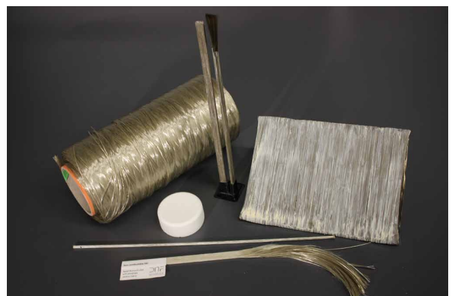
Basalt roving, CBPC matrix, pultruded profiles and wrapped sheet
