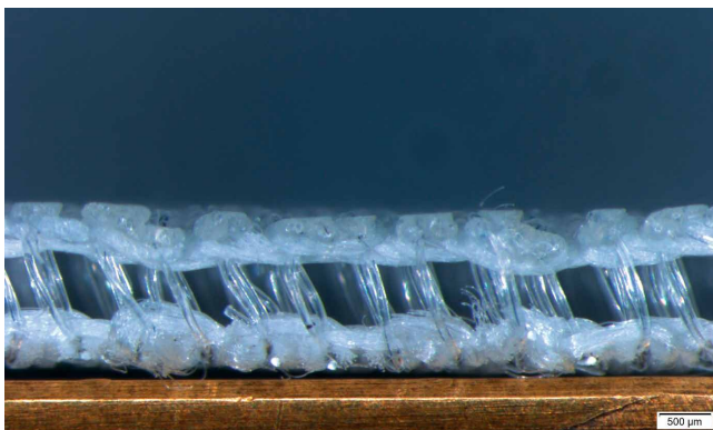
Pressure-resistant spacer fabrics are used as textile filling cores for vacuum insulation elements. The pore properties can be flexibly adjusted during the knitting process by selecting the yarn and weave.
