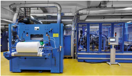
Carbon and natural fiber enabled 1,000 mm needle felt line
