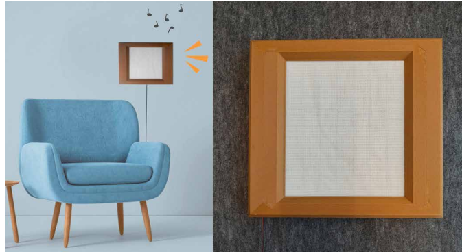
Left: The textile speaker can be hung on the wall like a picture frame and subtly fill the room with sound. Right: Developed speaker.
