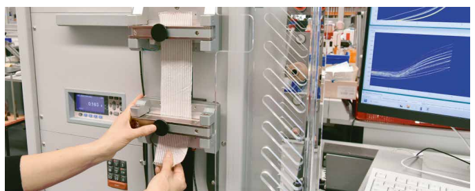
Measuring device for determining the electrical resistance along the force-strain curves
