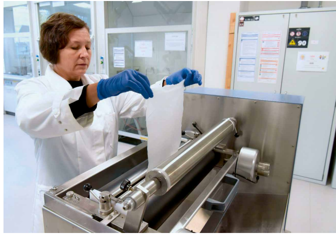
Equipment of a tissue on a laboratory padder
