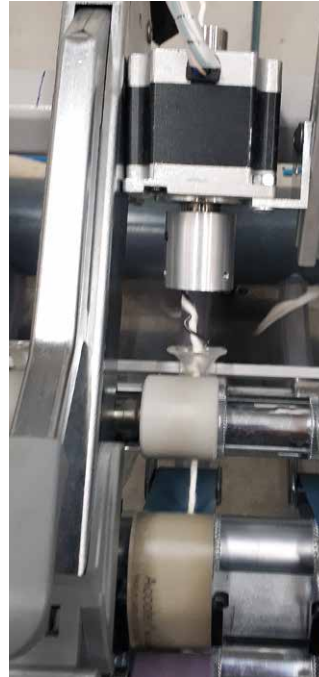
Twisting element in front of the drafting system of a ring spinning machine
