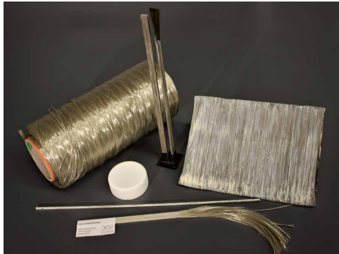
Basalt roving, CBPC matrix, pultruded profiles and a wound plate
