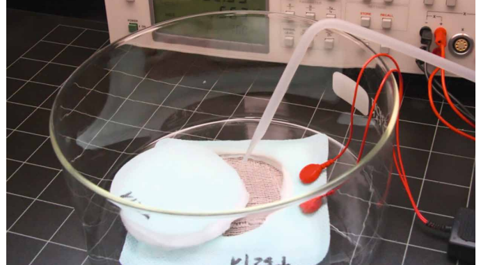
Determination of the moisture on the laboratory sample wound covering with sensor yarns
