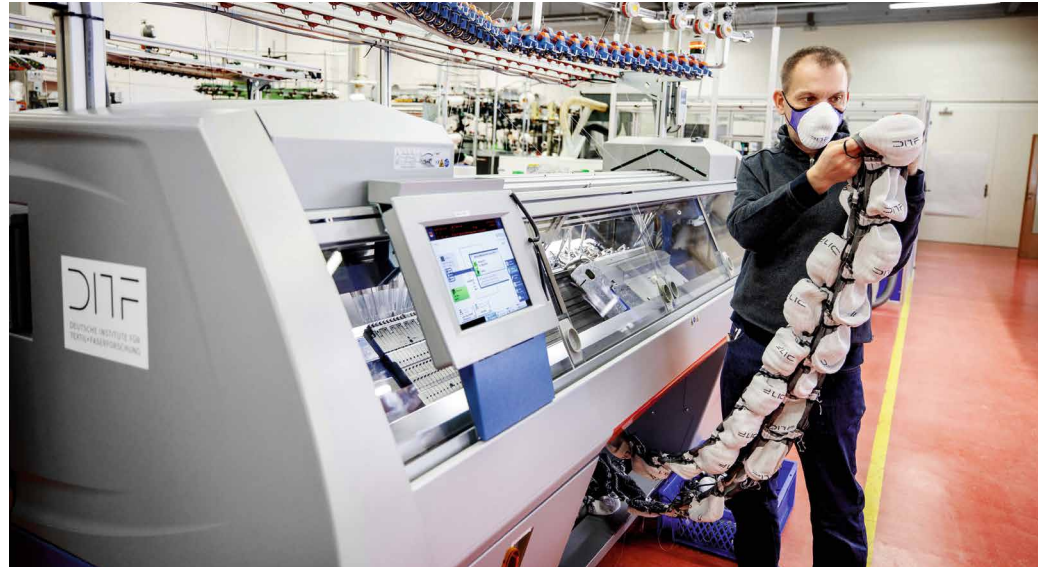
Everyday masks – finished in one operation from the knitting machine
