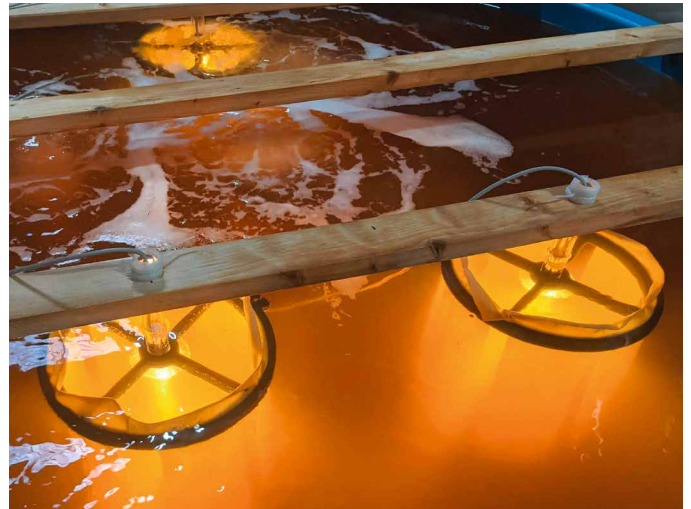
Algae production module (APM) with adapted carrier textiles
