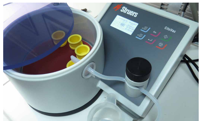
New at the DITF: Struers CitoVac vacuum embedding device
