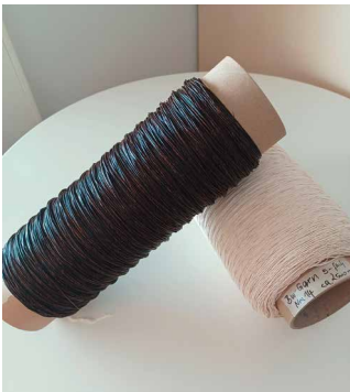
Cotton yarns: brown with lignin coating as a protective layer against degradation in the soil and white reference yarn without coating
