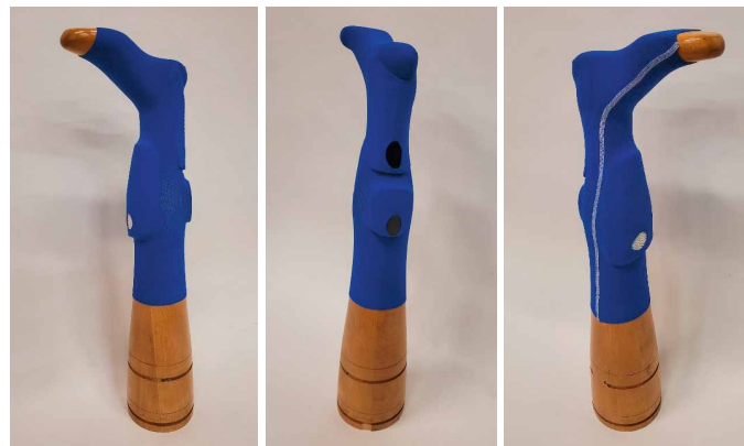
DITF development: soccer sock with mechanical absorber structures for the shin and calf as well as protectors to protect the ankle and Achilles tendon
