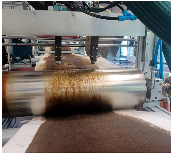
Cellulose-based nonwoven fabric is coated with the melted lignin compound as a protective layer against degradation in the soil
