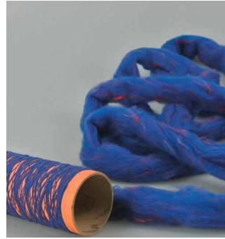
Yarn and knitted fabric made from 100 percent recycled aramid
