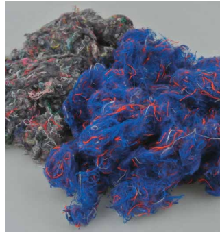
Used textiles after the tearing process. Back: Cotton, front: Aramid
