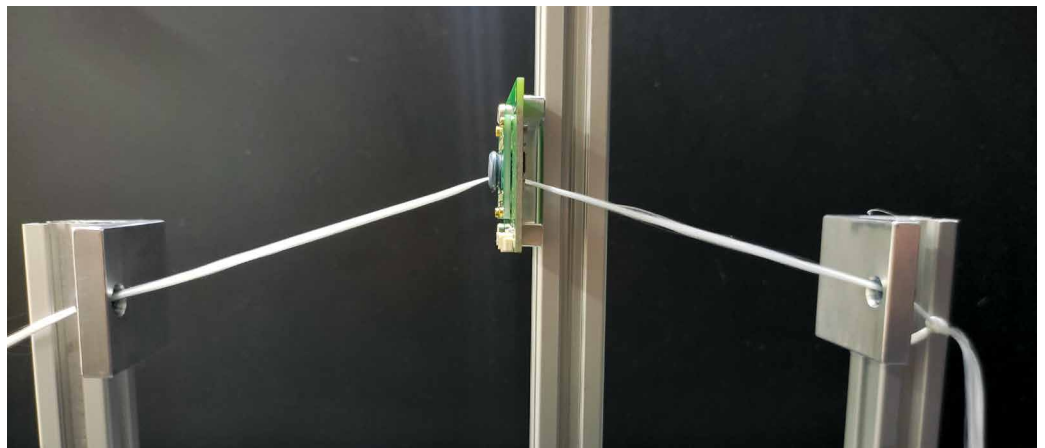
Structure of the thread tension sensor
