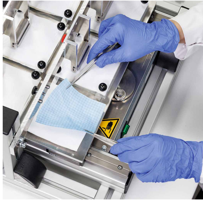
ReBa 2 testing device for determining the bacterial penetration of cleanroom garment textiles
