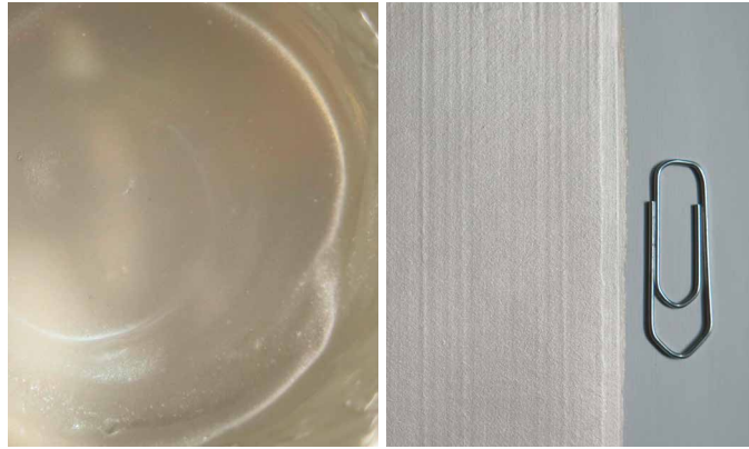
Electrically conductive printing paste (left), dried, conductive, elastic layer on textile (right)
