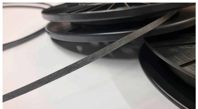
Developed "Infinity" rCF tape variant with trimmed tape edges
