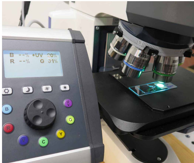
Carl Zeiss Colibri fluorescence device on Axioscope 5 reflected light microscope
