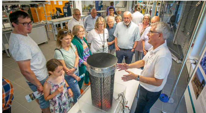
Spacer textiles collect water from the air: this fog catcher supplies people in dry areas with drinking water
