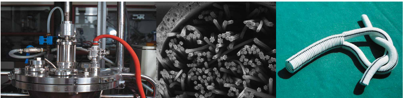
Left: Polymer lab: reactor for polymerization of resorbable polymers.
